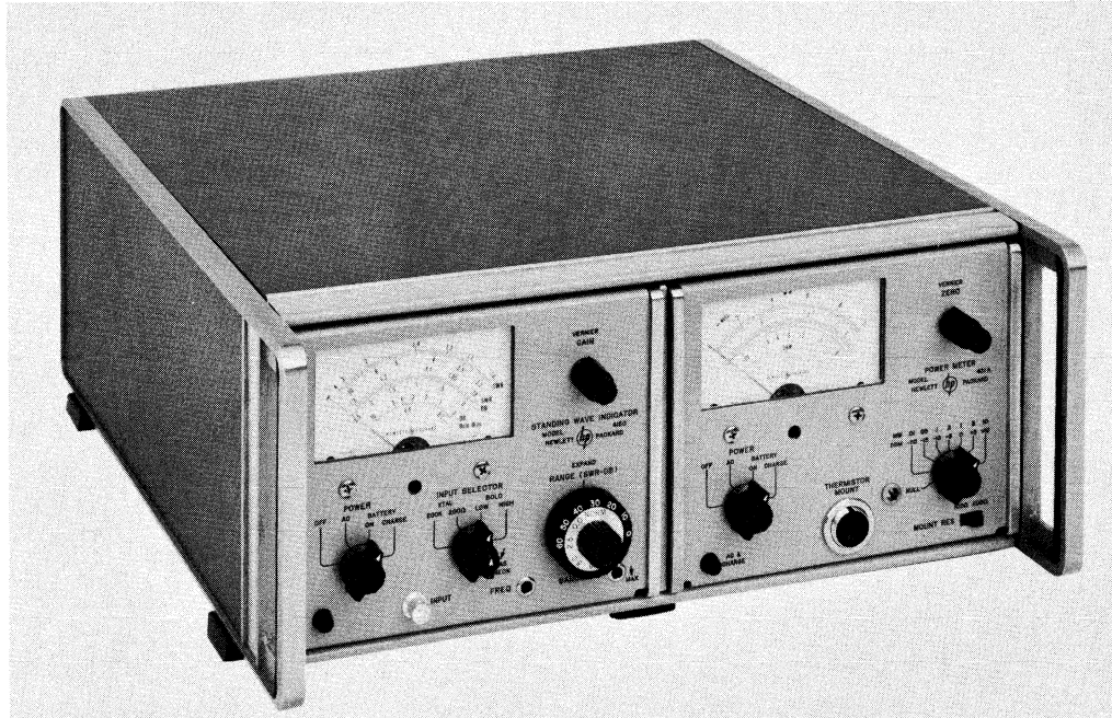
FIGURE 1-3 Two important microwave measuring instruments. The standing wave indicator (left) used when determining microwave reflections, and the microwave power meter (right).
